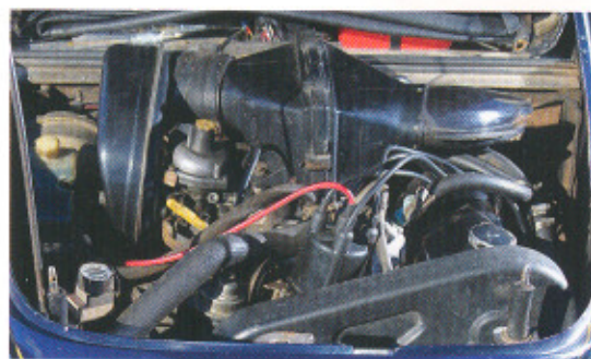
It's that 2300 overhead cam engine again.
