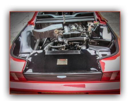
The engine is a turbo-charged 2 Litre, four cylinder Cosworth unit similar to the one fitted to the famous Sierra Cosworth. It develops 204 bhp at 6000 rpm and 200 lb ft of torque at 4500 rpm. Unlike any other mid-engined Supercar, the Solo's engine is mounted not only north-south but also asymmetrically in both vertical and horizontal planes in order to make room for the 4WD transmission, without adding length to the wheelbase.
