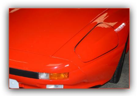
Smart lateral thinking resulted in the novel headlamp unit being engineered to swivel (rather than 'pop-up') which allows the Solo to maintain the exceptionally low Cd of 0.30
